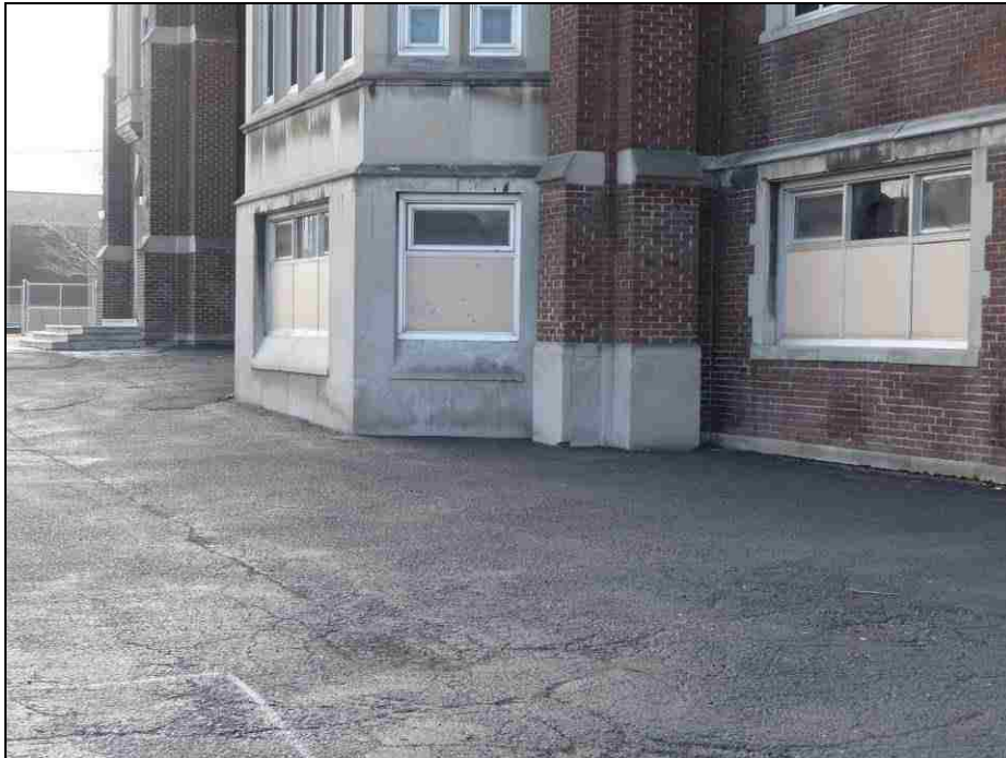
Figure 40. ES-03: School building architecture can create niches along corners and create unintended semiprivate spaces for children.
