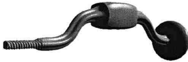
Figure 1.9. A Model Defined by Sweeping Primitives
