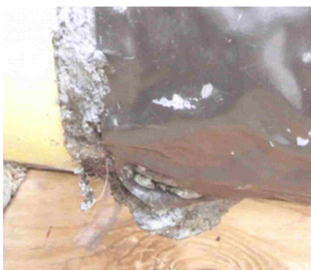
Figure 1.5 – Part 1, Calcareous Deposit Example –Shrink Sleeve & Coating Interface
