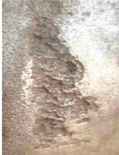
Figure 1.6 – Part 2, Calcareous Deposit Example –Shrink Sleeve & Coating Interface 12
