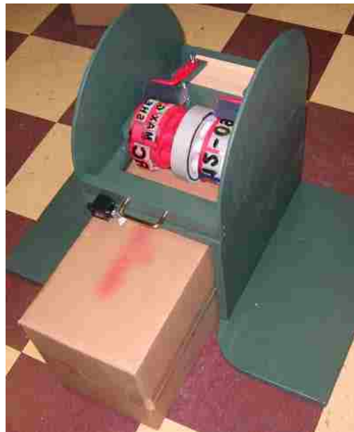
Figure 4.7. Embodied design for the box-labeling device (cover removed to show internal components).
