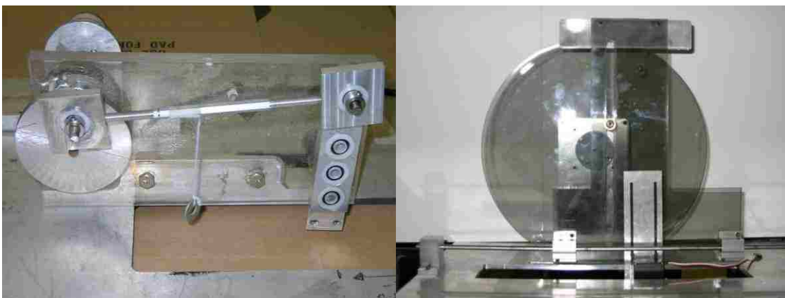
Figure 3-2: Flapping (left) and plunging (right) mechanisms.
