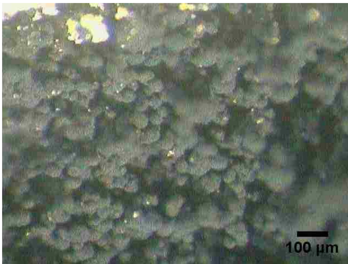
Figure 4.10. Optical microscope image of pyrolytic soot deposit on center of the anode after cell operation in propane.
