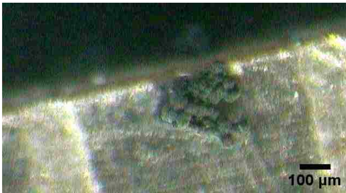
Figure 4.11. Optical microscope image of pyrolytic soot particle from anode, which rubbed off onto the edge of a 1mm ruler.
