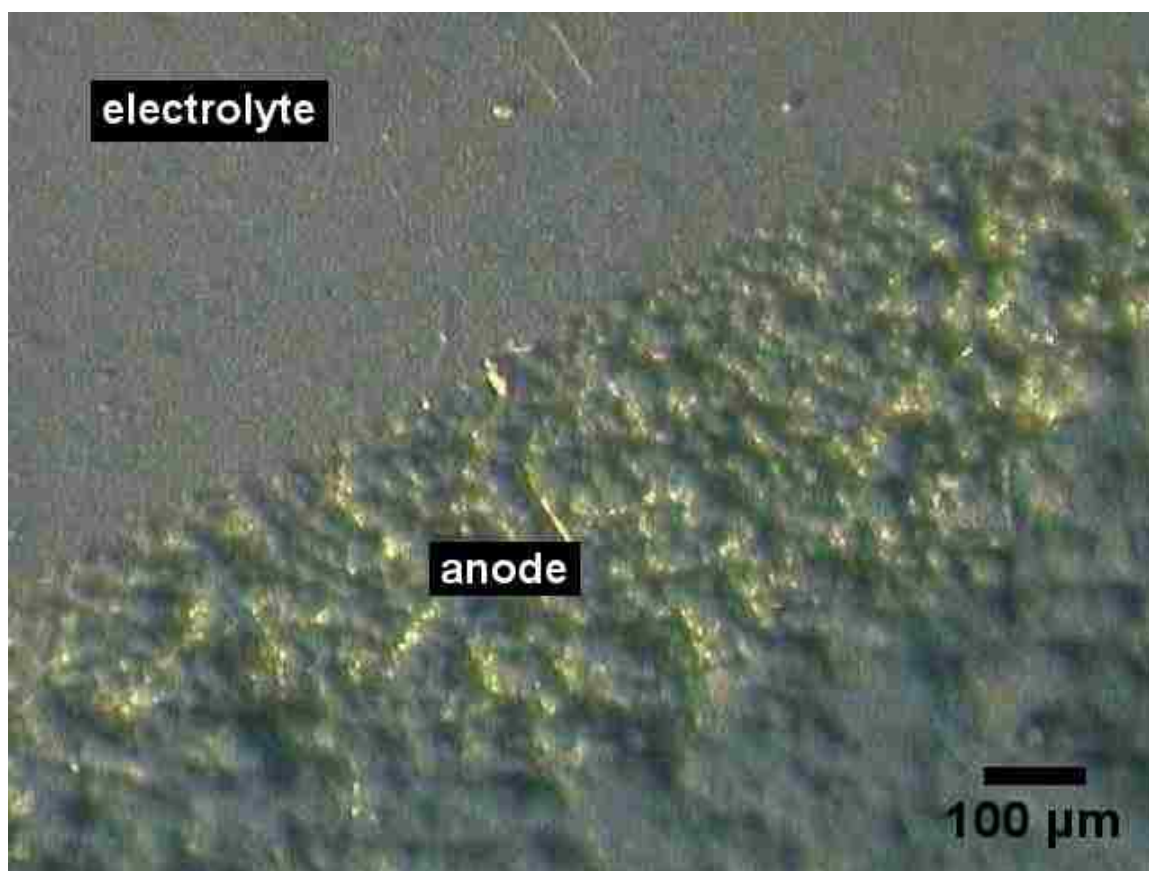
Figure 4.8. Optical microscope image of thin single-dip acetylene soot deposit on electrolyte and edge of the anode.
