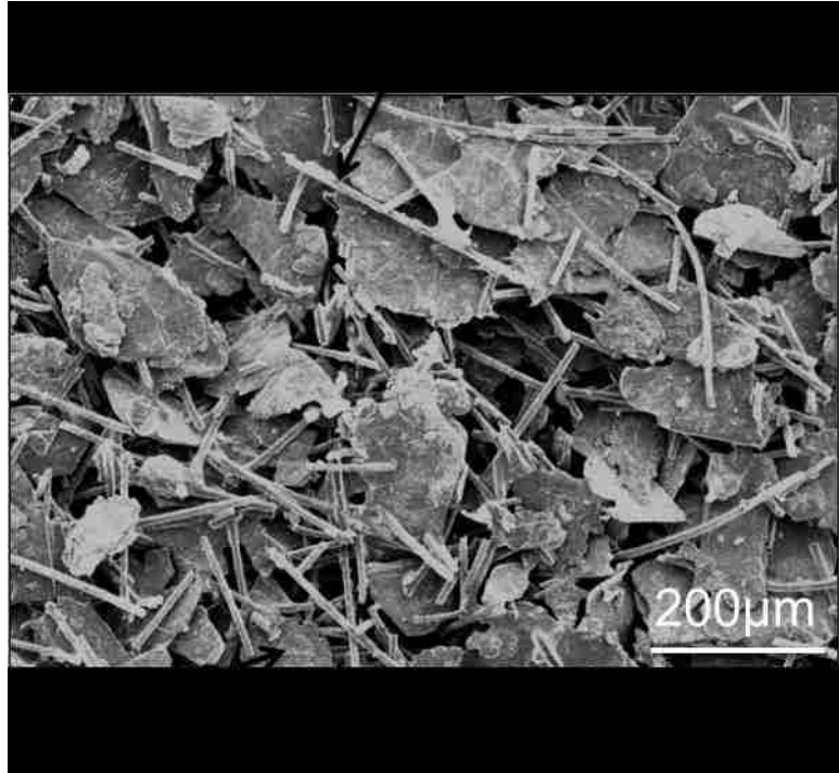
Fig. 6 Microstructure of a brown part made from 25vol% CF, 40vol% NG and 35vol% binder.
