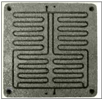
Fig. 11 Bipolar plate with a serpentine flow field (active area: 50×50 mm 2 , thickness: 4 mm, channel width: 1.5 mm and depth: 1.5 mm).
