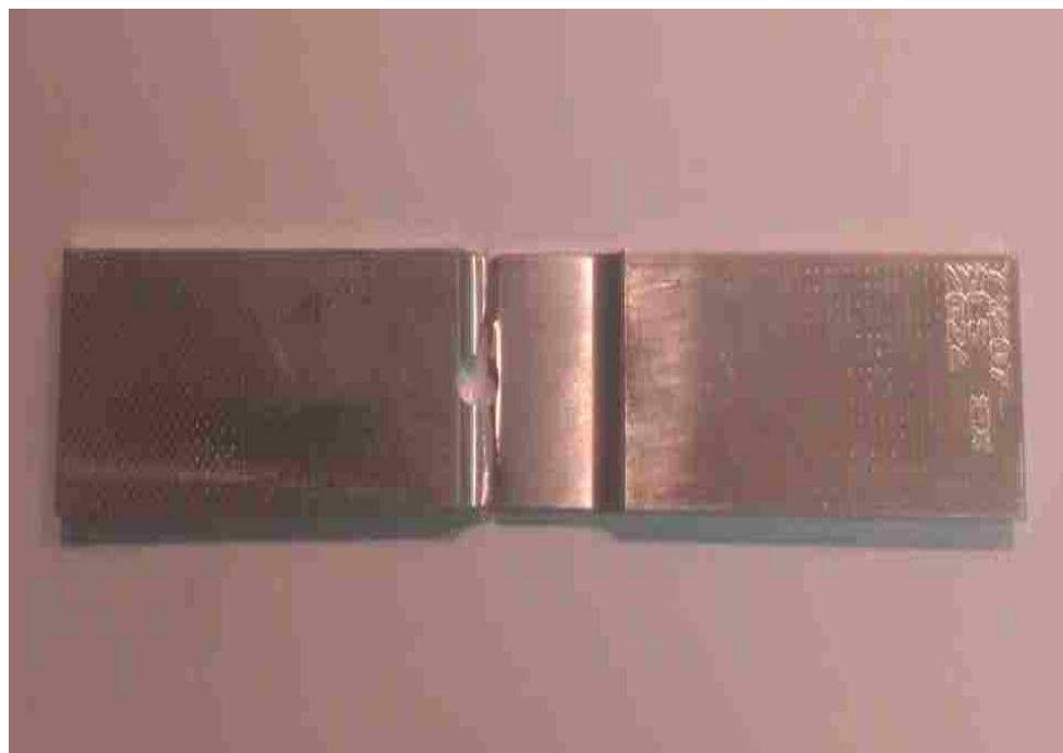
Figure B.12. Open Hole in Radius Test Specimen -6 Post-Test Picture
