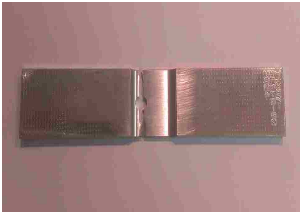
Figure B.11. Open Hole in Radius Test Specimen -5 Post-Test Picture
