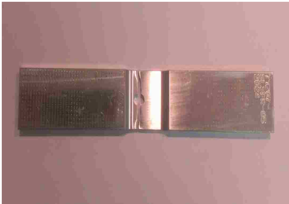
Figure B.9. Open Hole in Radius Test Specimen -3 Post-Test Picture
