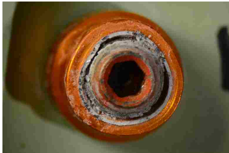
Figure 4.23. Post-Test Stress Corrosion Fastener 11 Collar
