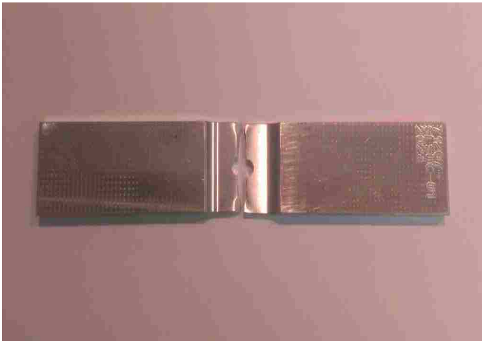
Figure B.8. Open Hole in Radius Test Specimen -2 Post-Test Picture
