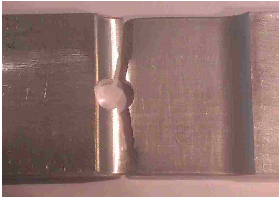
Figure 4.12. Close-Up Picture of Post-Test Open Hole in Radius Test Specimen -6
