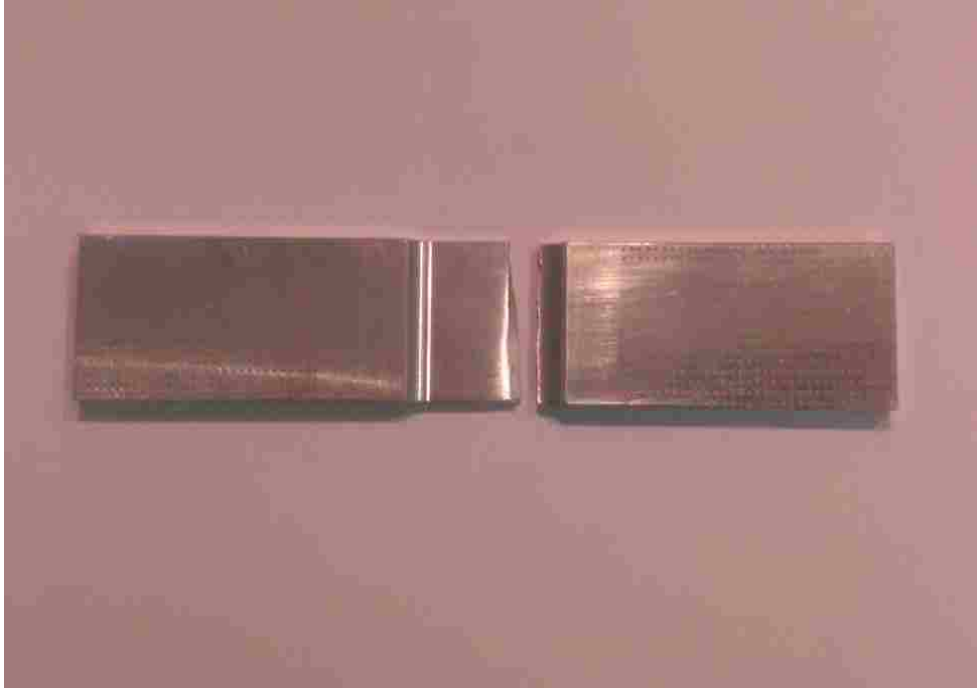
Figure B.7. Open Hole in Radius Test Specimen -1 Post-Test Picture
