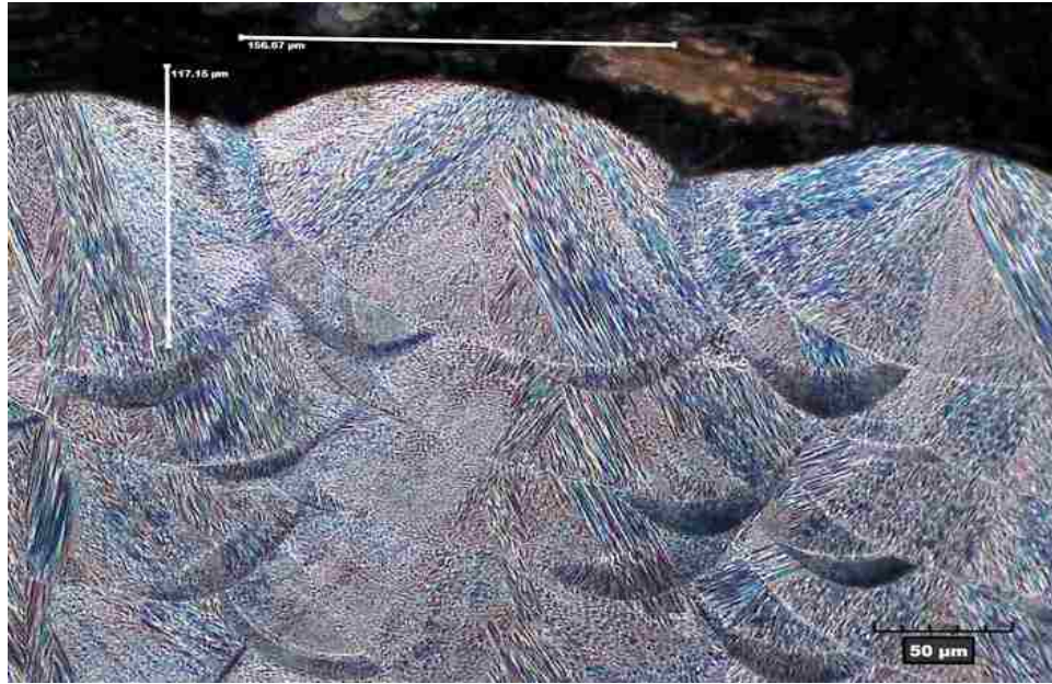
Figure 4.7. Top Layers of Structure Built with Laser Power 150W and Point Distance 60µm
