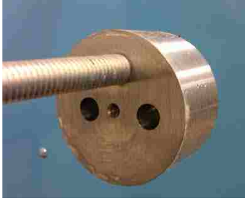
Figure 11. Backing plug used to determine microphone calibration gain and phase angle correction factors.
