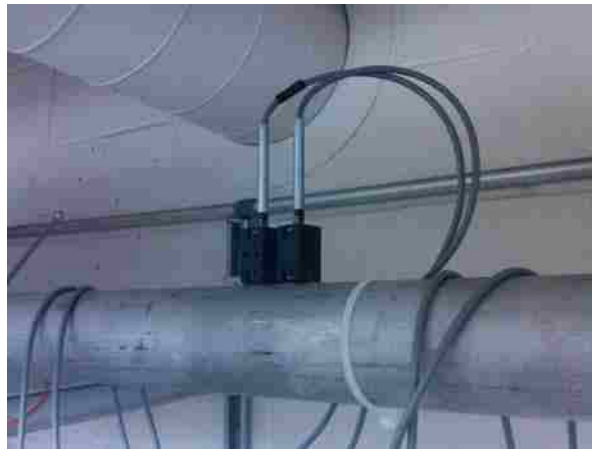
Figure 10. Microphones mounted in the side of the tube in the measurement location.
