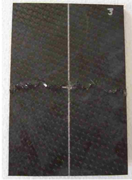
Figure 8. Front View of MTM45-1/CF2412 Composite Sample under CAI Testing
