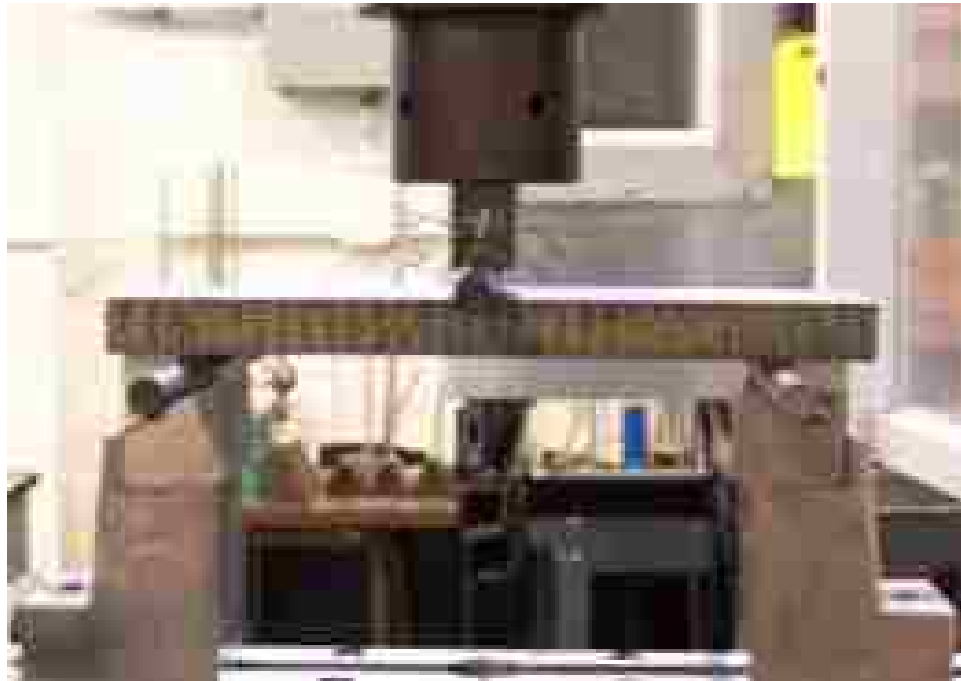
Figure 8. Three Point Bending Test Set-up
