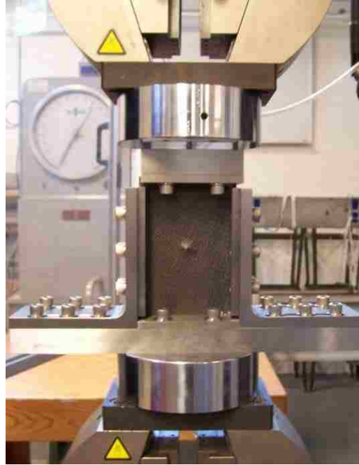
Figure 18. CAI Testing Set-up
