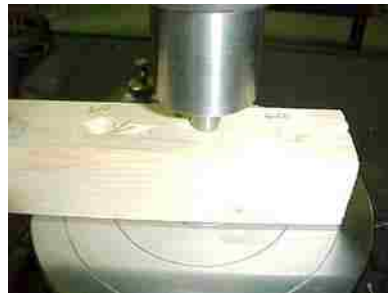
Figure 3.4. Janka Hardness Testing
