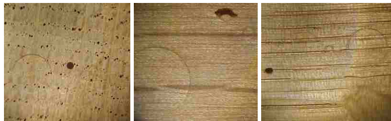
Figure 3.2. Indentation Marks in Longitudinal, Radial, and Tangential Directions
