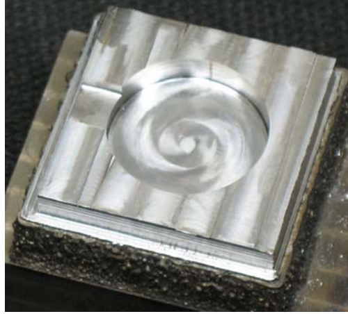
Figure 11 Deposited part using the adaptive toolpath pattern after top surface machining.
