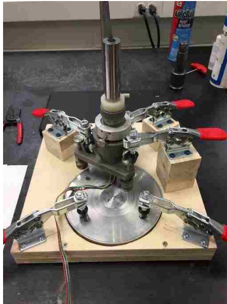
Figure 2.14 Hole Drill Fixture
