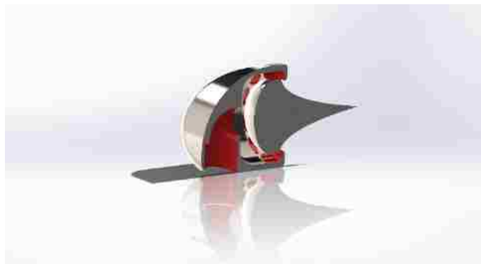
Figure 3.5 Aerospike Nozzle Section View
