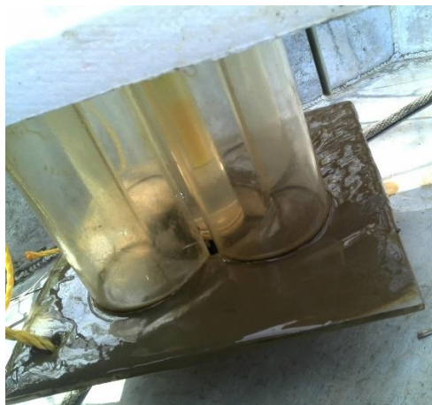
Figure 2.2. Quatrefoil light trap post deployment. The light stick in the center lures aquatic organisms which become trapped in the clover shaped outer tubes.
