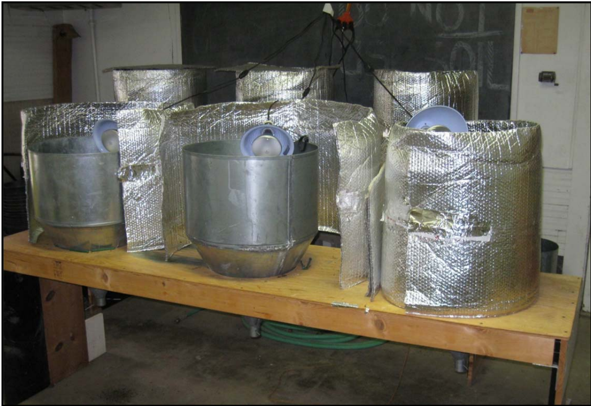
Figure 7. Large Berlese Funnels with brooder lamps that desiccate salvinia samples and allow the retrieval of live C. salviniae weevils for dissection or other research purposes.
