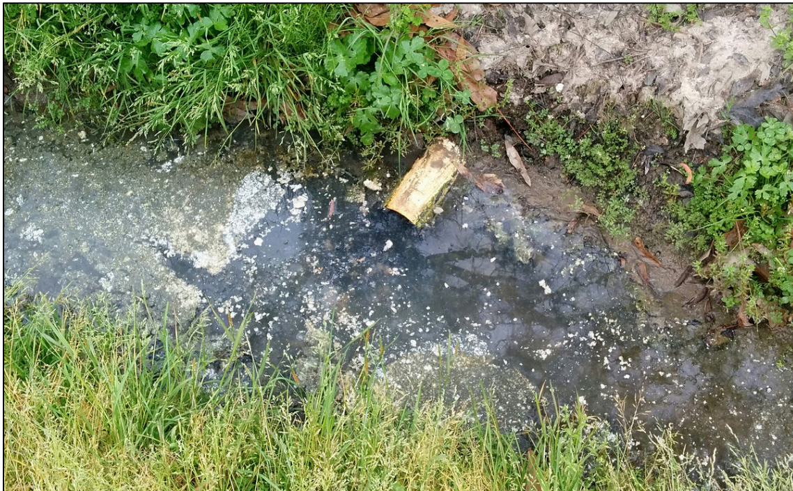
Fig. 9. Picture of a water quality sampling site: drainage ditch with white septic outlet pipe. Lovett Rd, East Baton Rouge Parish, LA.
