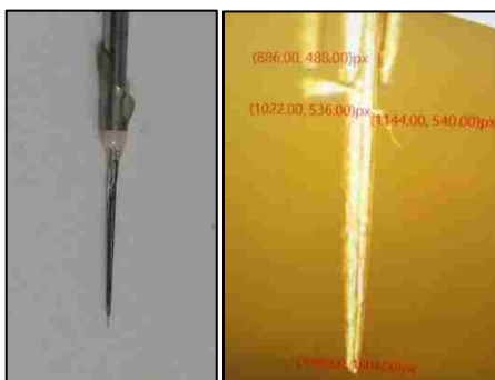
Figure 3.3. Probe Tip (a) and Probe Tip Under Microscope (b)
