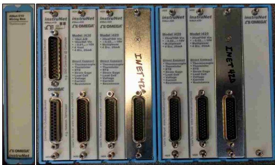
Figure 3.8. Portable DAQ for Conductivity Probe iNET-510 (a) and iNET-430 (b)
