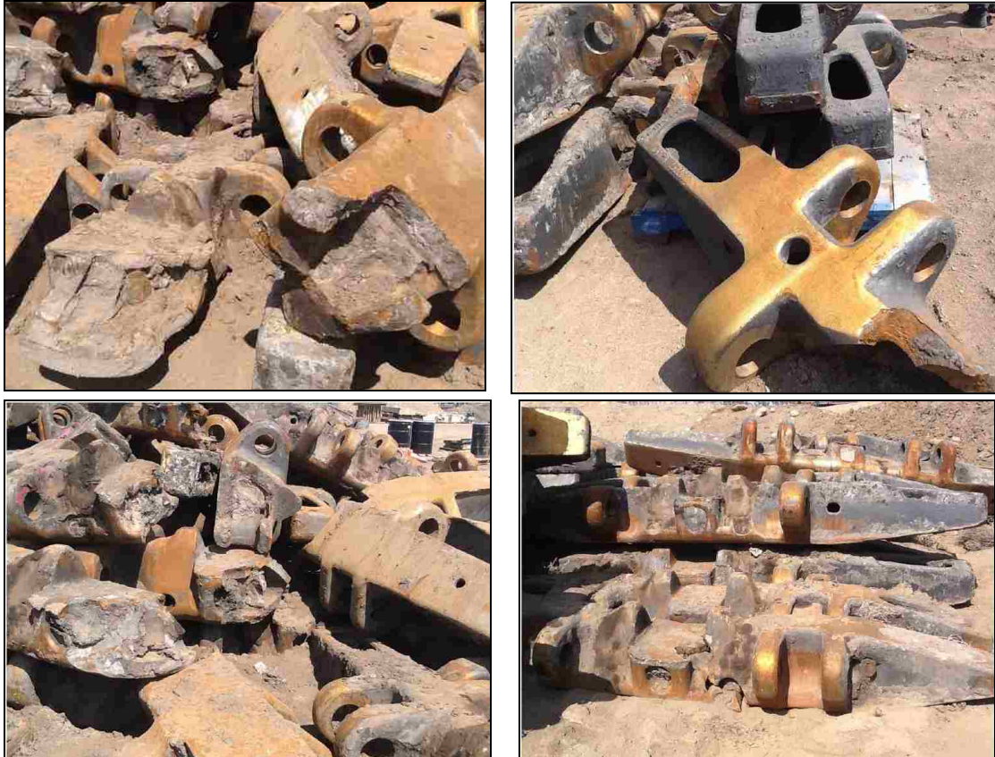
Figure 1.6. Wear and Fracture in Crawler Shoes (Syncrude, 2014)
