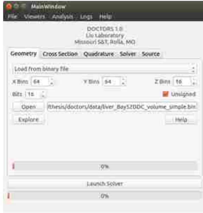
Figure 4.9. The geometry selection tab. The user must first specify the dimensionality of the voxel phantom and then load it from a binary file.
