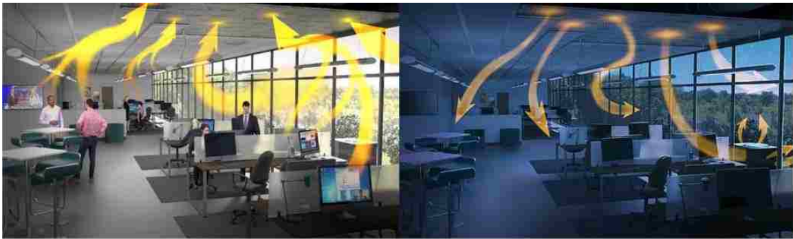
Figure 1.16. PCMs storing heat (left) and releasing heat (right).
