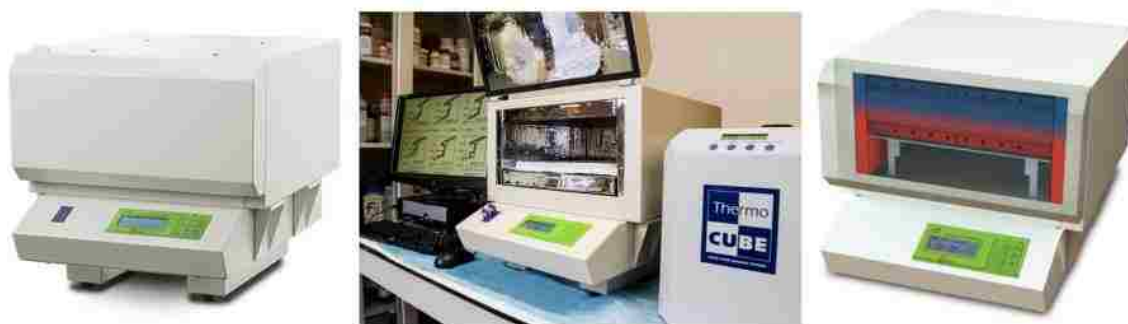
Figure 2.2. The guarded parallel-plate heat flow apparatus using Fox314 TA instrument [86]
