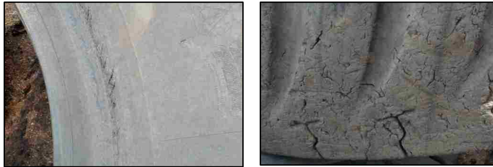
(b) Tread Lug/Groove Cracking
