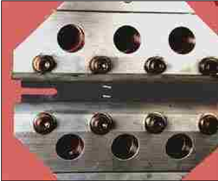
Figure 5.14. Planar Tension Specimen [113]
