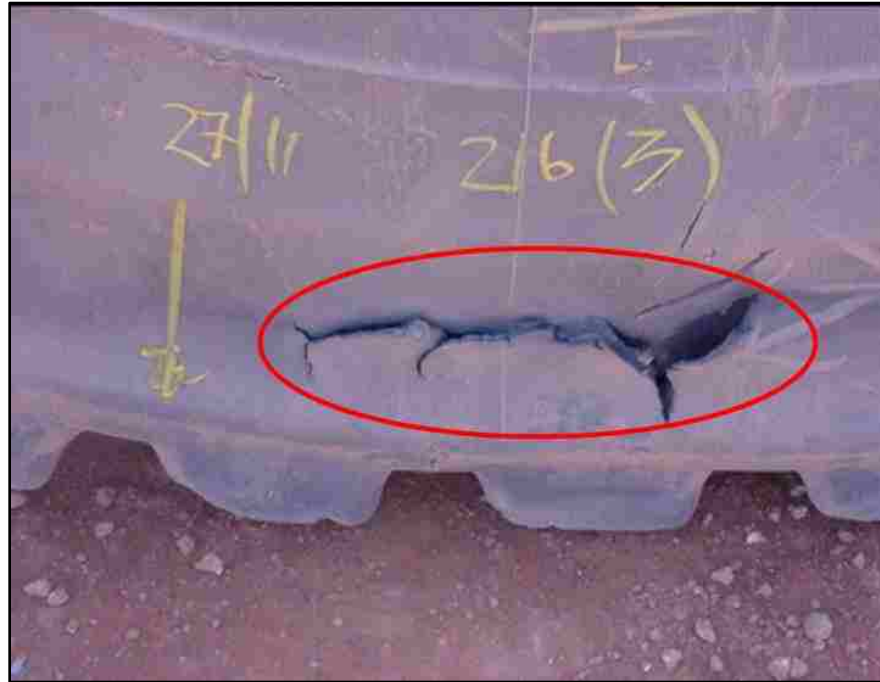
Figure 1.3. Mechanical Separation in a 55/80R63 Tire [10]
