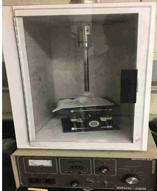
Figure 5.1. Vibra-cell sonicator for stabilizing nanoparticle suspensions.
