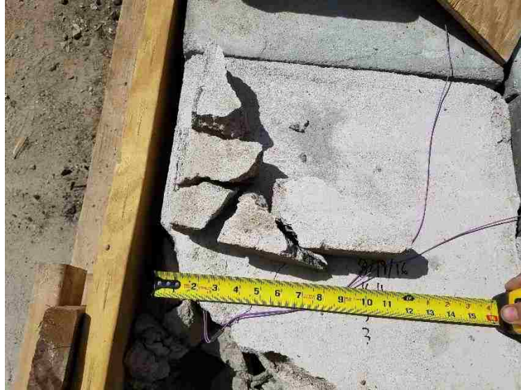
Figure 6.13. Test 13 3" 50%/50% Mix Cap Surface Breakage
