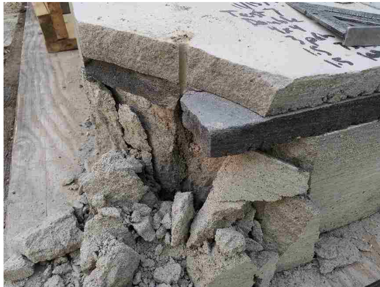
Figure 6.21. Test 21 2-Layer Cap Side Profile
