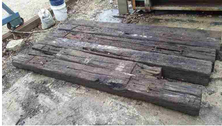
Figure 4.1. Test Bench Railroad Tie Configuration (Note difference in length on second tie)
