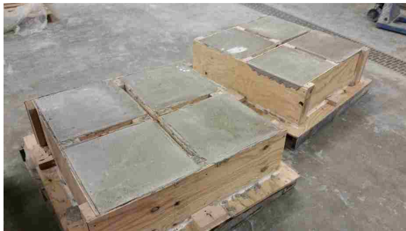
Figure 4.3. Cast Test Specimens in Constructed Forms
