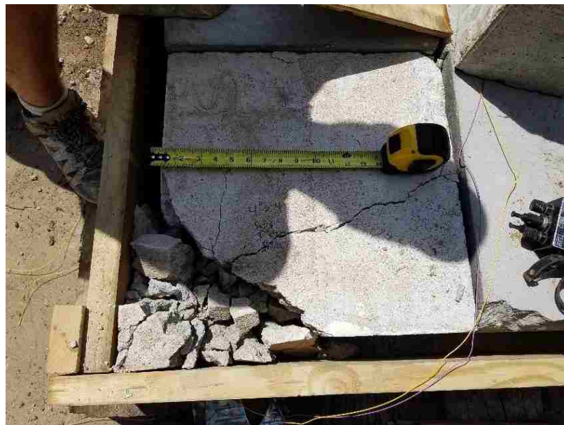
Figure 6.12. Test 5 Solid Block Surface Breakage
