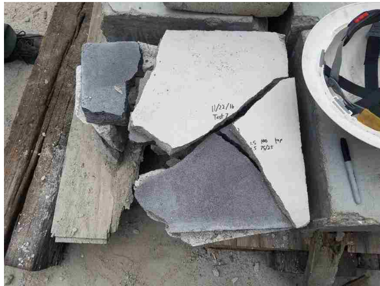
Figure 43 Middle Layer and Block Breakage Test 30
