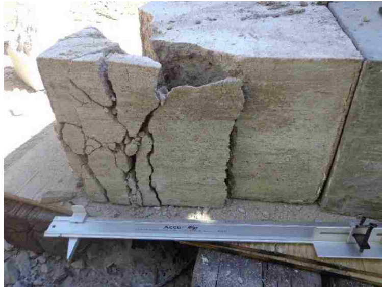
Figure 4 Side Breakage Test 2
