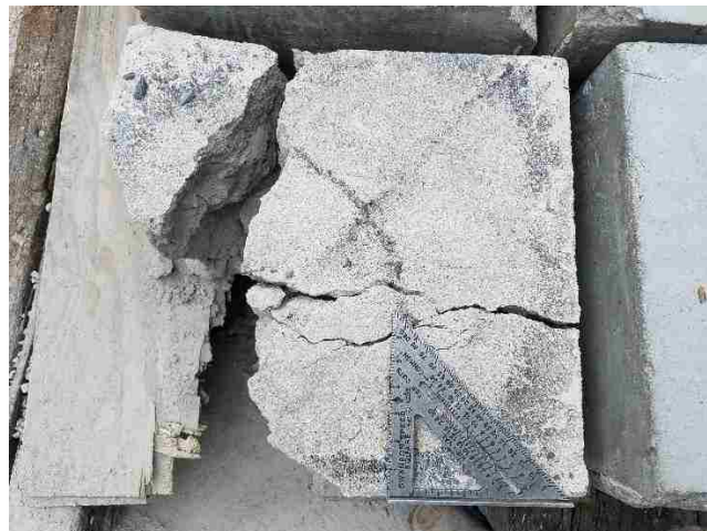
Figure 5.8. Substrate Block Fractures 2-Hole, Test 30 11/22/16
