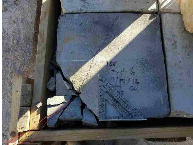
Figure 28 Surface Breakage Test 20
