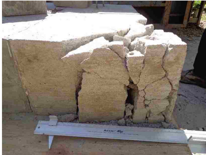
Figure 2 Side Breakage Test 1
