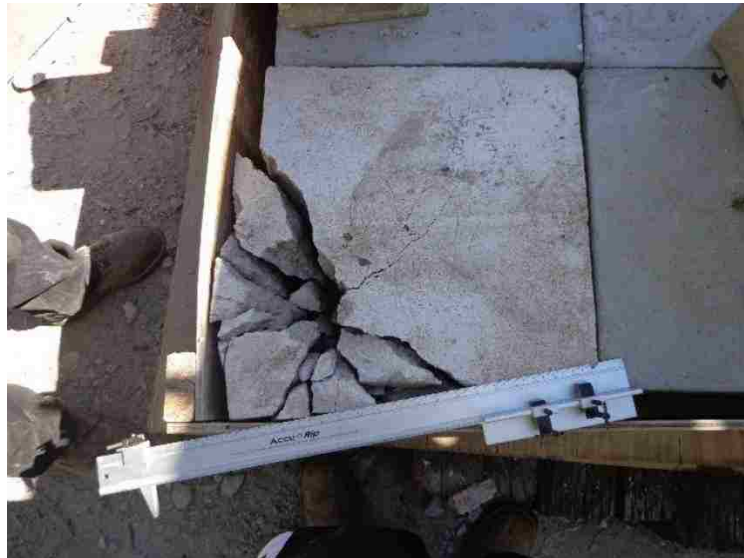
Figure 3 Surface Breakage Test 2
