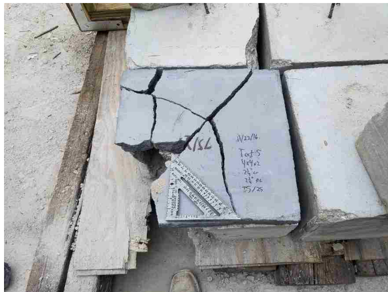
Figure 39 Surface Breakage and Annular Fracture Test 28
