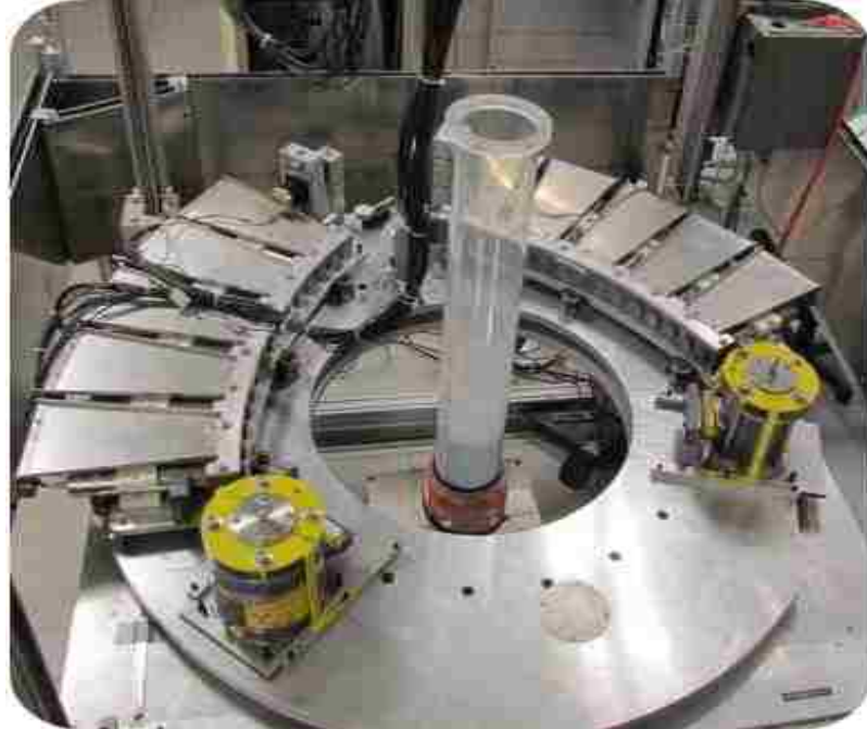
Figure 3.5. Photograph of the DSCT technique, and 6-inch spouted bed inside the setup for scan.
