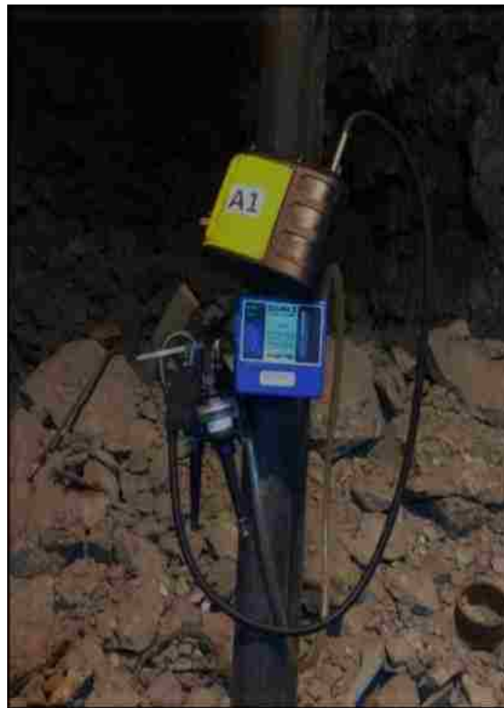
Figure 3.5 DPM monitors installed in the mine Y
