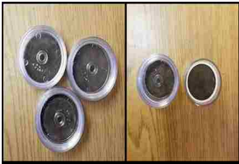
Figure 9.4 Moderately contaminated DPM cassettes
