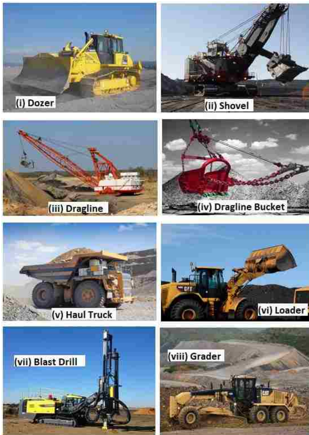
Figure 4.3. Mobile mine equipment object classes [149, 150]
