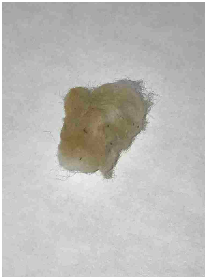
Figure 2.4. Post-blast Residue from Binary Explosive Collected onto a Cotton Ball
