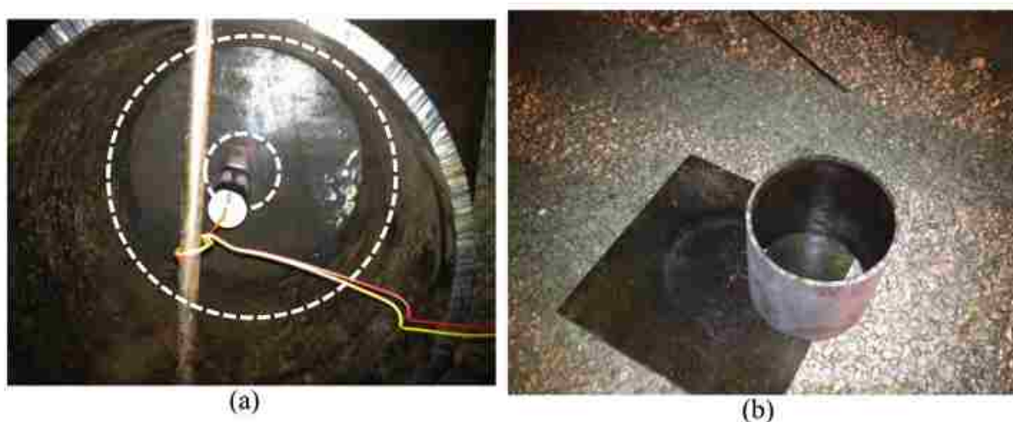
Figure 4.1. Single Element Binary Post-Blast Test Showing the Charge Contained within the Steel Cylinder. Denoted (a) and the Same Cylinder after Detonation, with Post-Blast Residue Apparent at the Center (b). A Representative Sampling Path is Indicated by the Dashed Circles in Figure 4.1a
