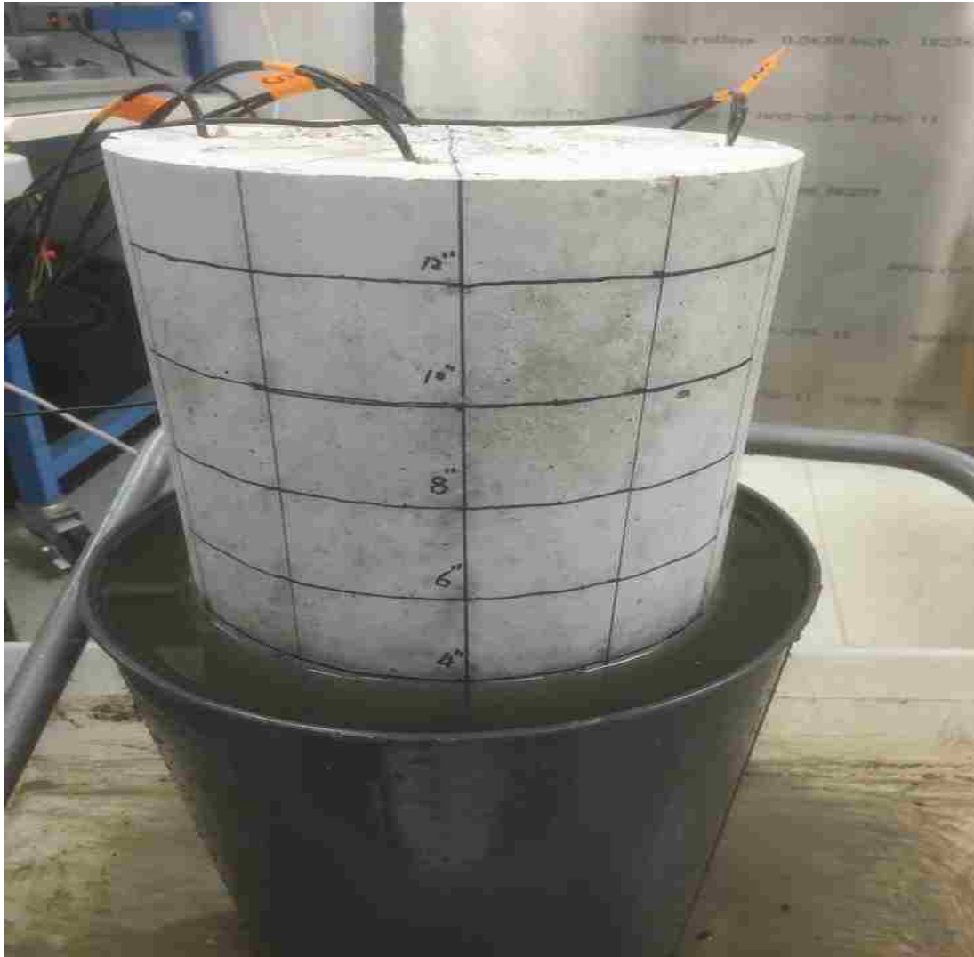
Figure 5.5 Model concrete pile submerged in water
