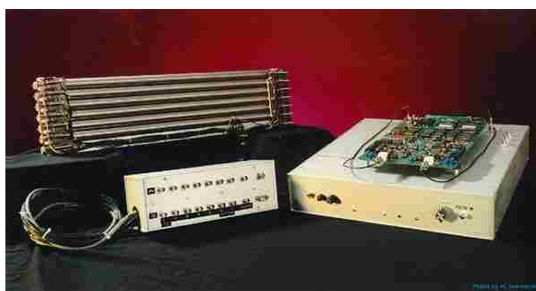
Figure 2.13. The neutron detector array at NPDF, NCSU[37]
