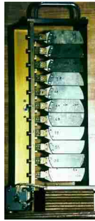
Figure 2.12. Vertically focusing Ge wafer monochromator at HRPT[32] .
