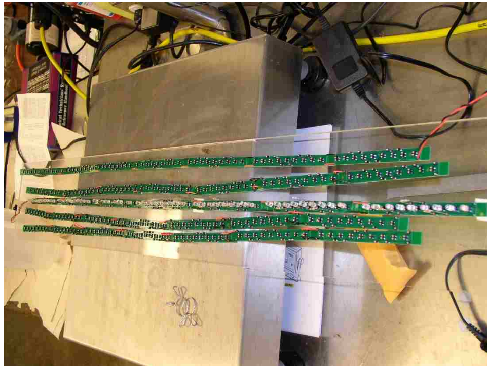
Figure 3.22. Photograph of light strips composed of the nine-LED PCB boards.
