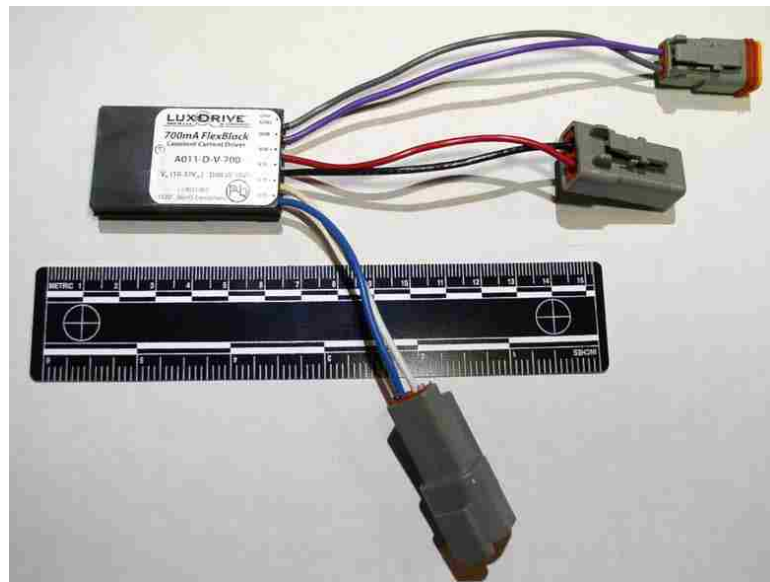
Figure 3.27. Photograph A011 FlexBlock modified for use within the experimental set-up for blue LEDs used in the capstone experiment
