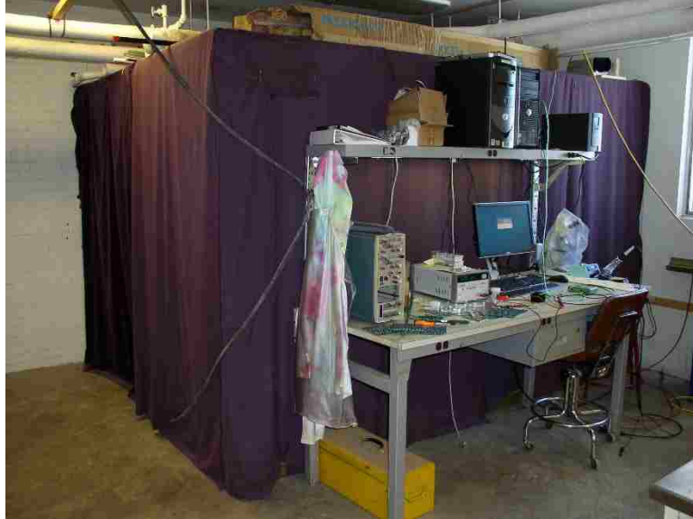
Figure 3.19. Finished darkroom with black-out curtain applied.
