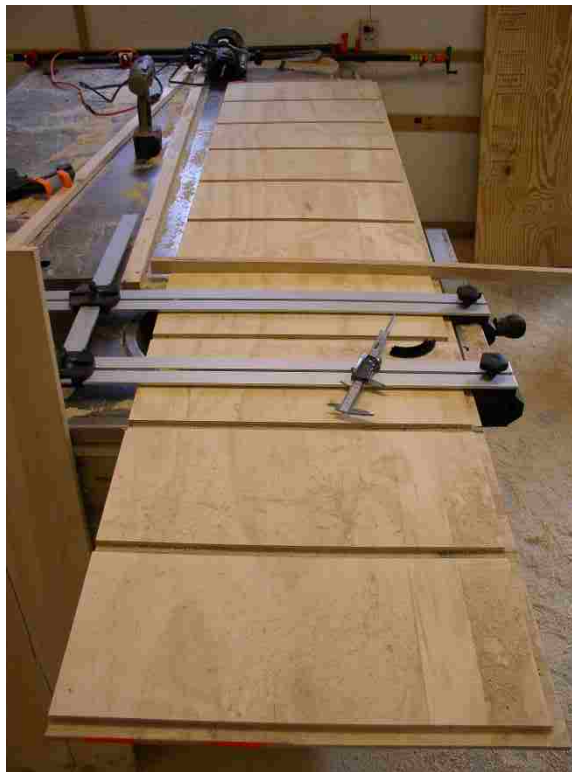
Figure 3.15. Picture of the dado and rabbet joinery used to construct a light-tight experimental test cabinet.
