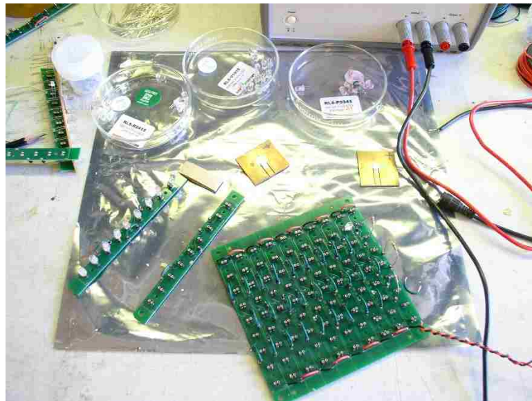
Figure 3.23. Photograph of nine-LED PCBs and a ninety-LED PCB array built by the researcher.
