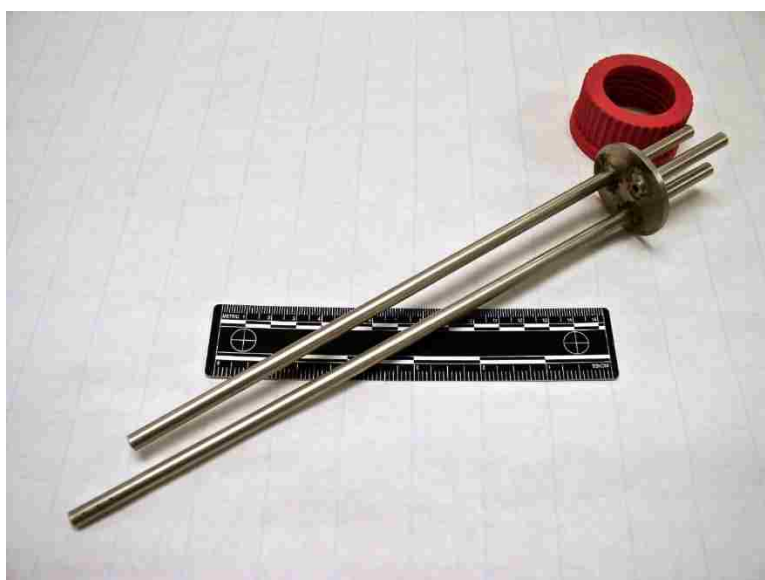
Figure 3.30. Stainless steel experimental port assembly for algae growth experiments reported in the capstone study.
