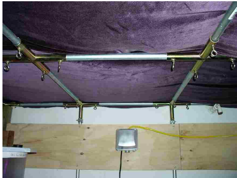
Figure 3.18. Picture of framework built around the experimental cabinet to support theater curtain.
