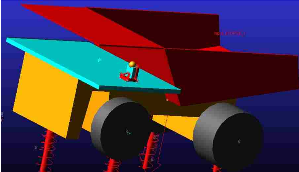
Figure 6.2 A 3D view of the virtual prototype model of the CAT 793D dump truck in ADAMS/View.
