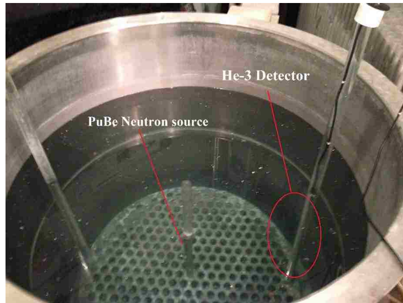
Fig. 4. Picture of ^3\text{He} detector neutron measurements in subcritical assembly
