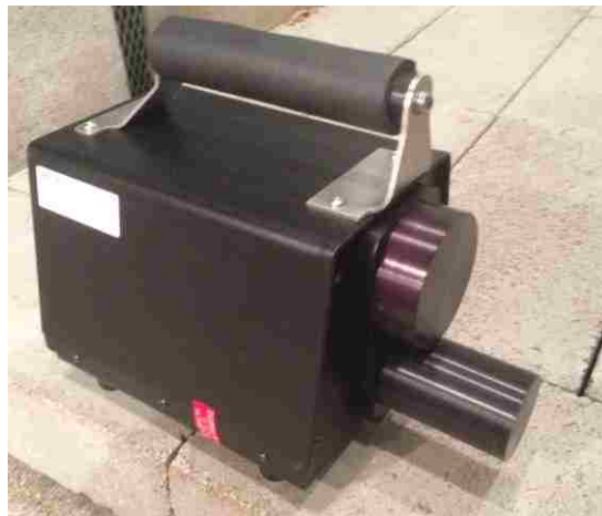
Fig. 1. N-Probe fast and thermal neutron spectrometer [9].
