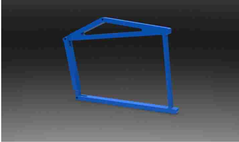
Figure 4.5. Solid Model of a Compliant Mechanism with One Fixed-Fixed Segment
