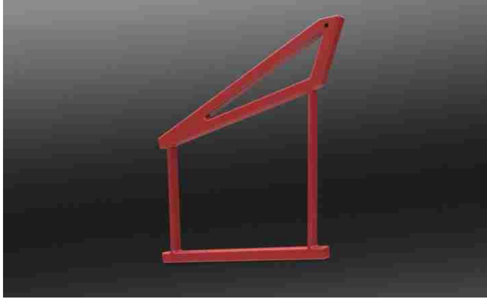
Figure 4.7. Solid Model of a Compliant Mechanism with Two Fixed-Fixed Segments
