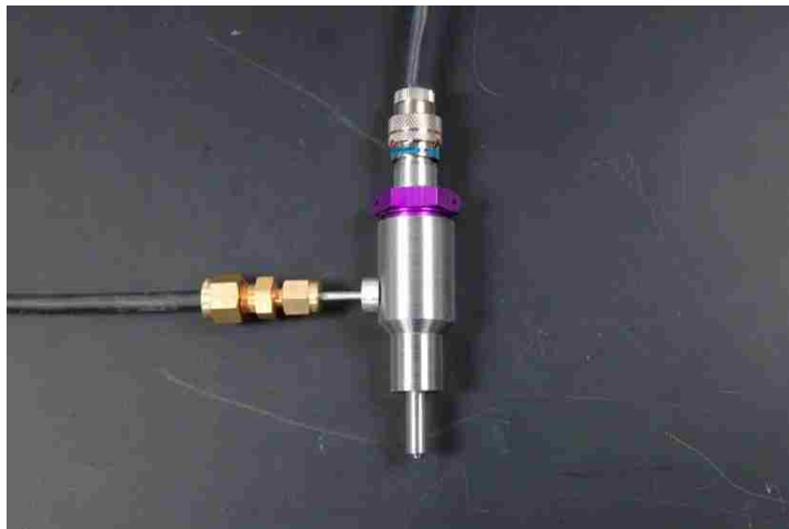
Figure 3.2. Residual gas injector used for in-cylinder species addition.
