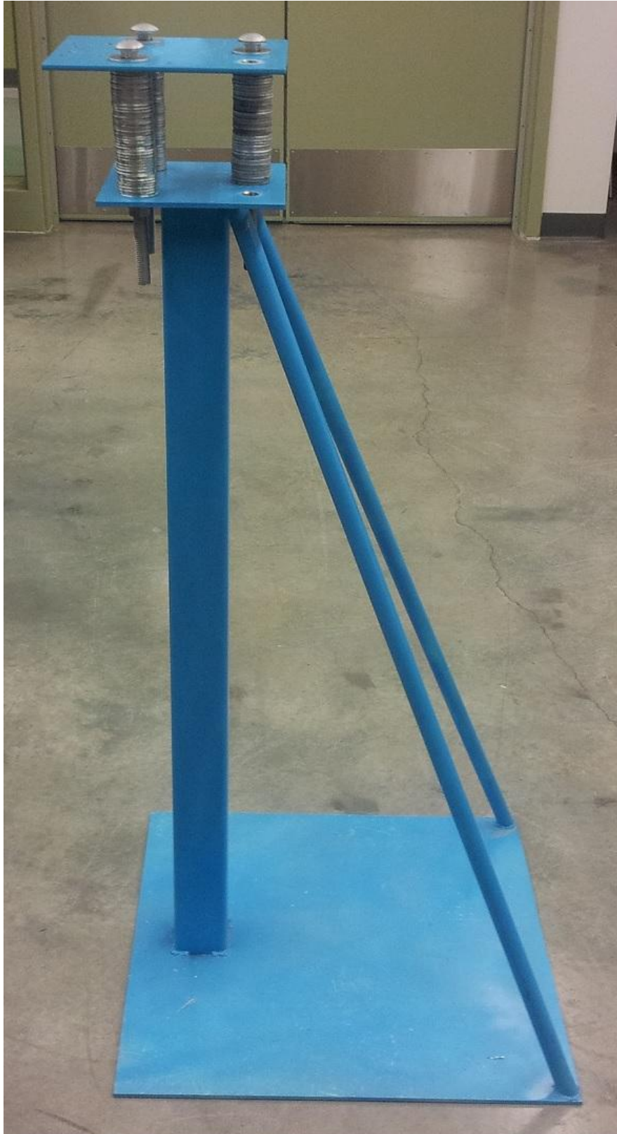
Figure 5.4 – Test Stand used to Attach Blade Fixture and Allows for Single Point Bending to be Applied from MTS 810 Machine
