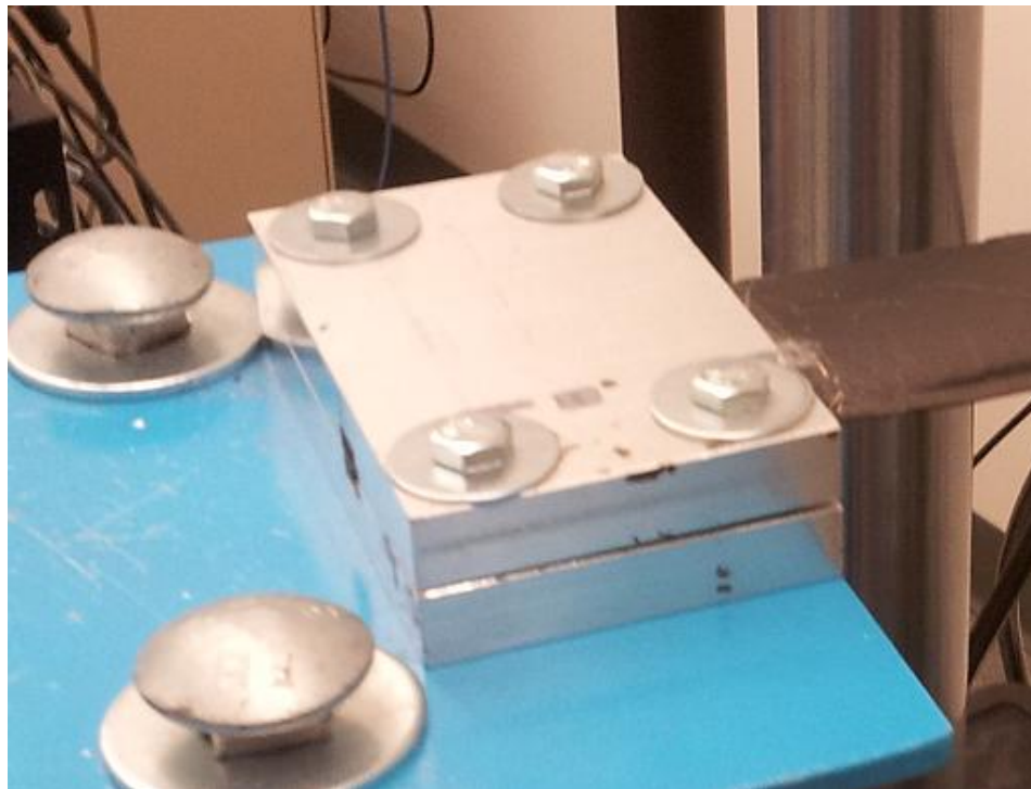
Figure 5.3 – Fixture used for Blade Design 1.1 and 1.2 that Isolates the Blade Span
