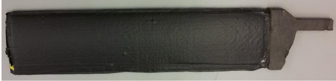
Figure 3.6 – Composite Blade Design 1.2 with Metal Epoxy Tabs and Three Extra Layers of Pre-Preg Wrapped and Cured to Blade Span
