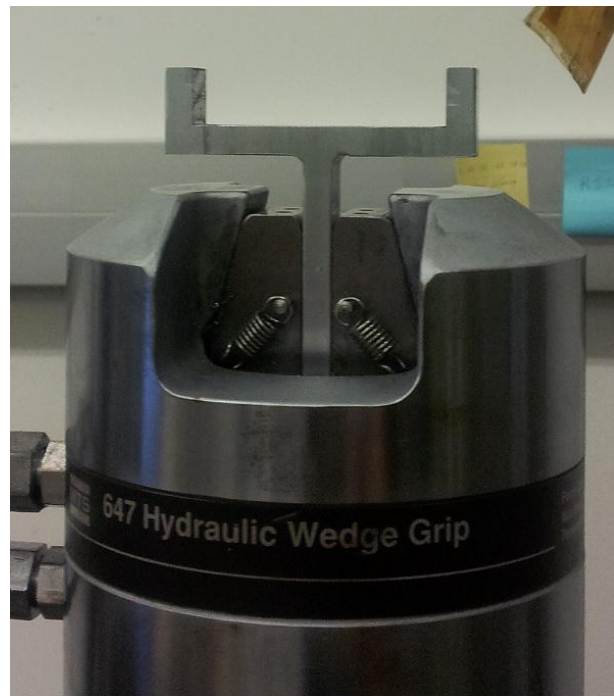
Figure 5.6 – Centric Fixture used in Conjunction with Blade Design 1.1 and 1.2 to Prevent Blade Twisting
