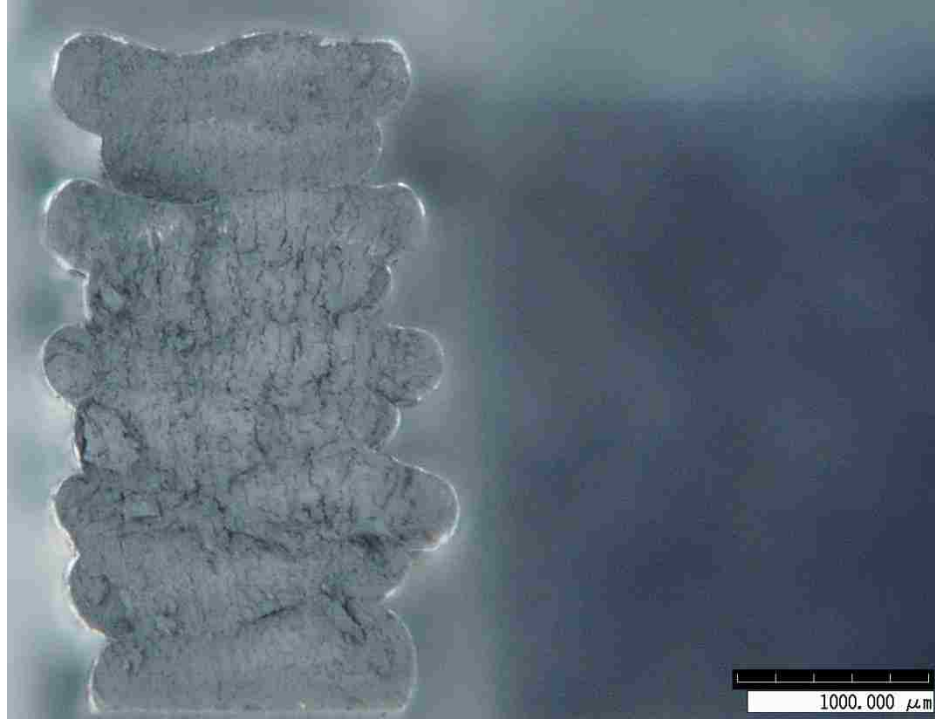
Figure 2.5 Thin-wall Cross-section Frozen at -20^{\circ}\text{C} , on an Aluminum Plate
