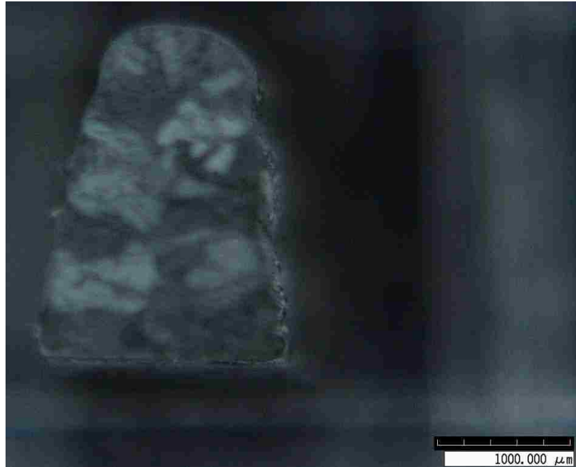
Figure 2.3 Thin-wall Cross-section Frozen too Slowly
