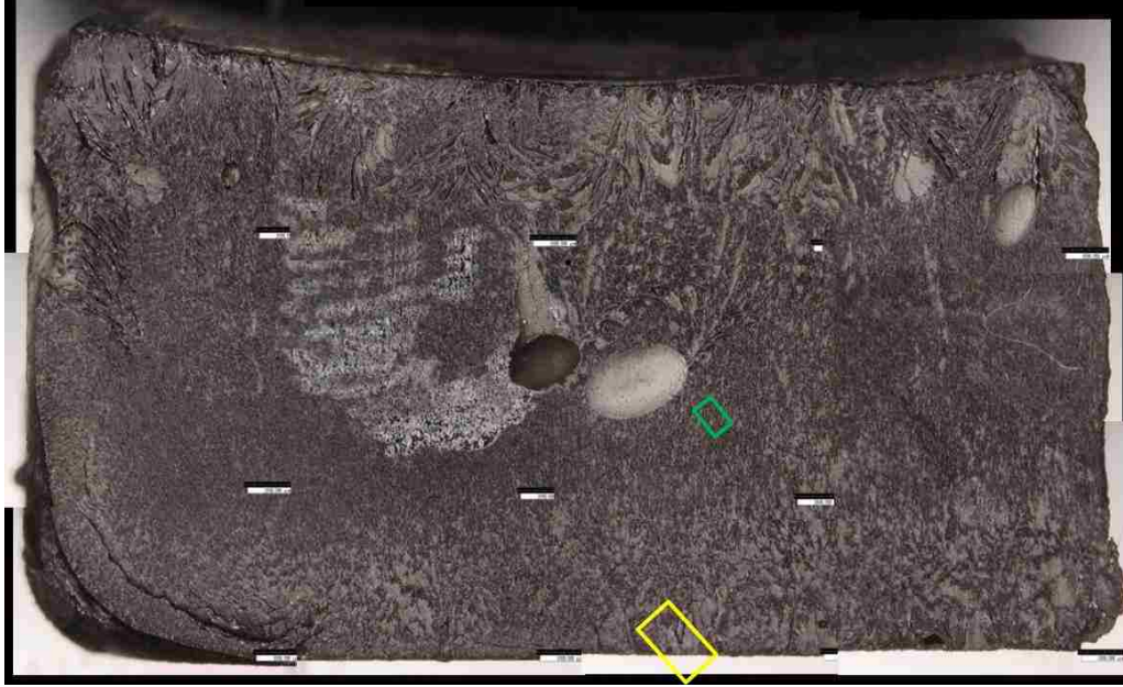
Figure 3.5 50x Zoom Map of Freeze-cast Bar #2 (Table 3.3) from the 10 wt% by Water Glycerol Group
