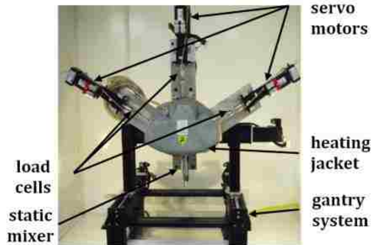
Figure 1.1 The Triple-extruder Freeze-form Extrusion Fabrication (FEF) Machine Inside the Environmental Chamber
