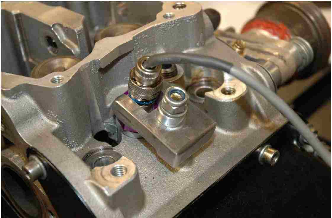
Figure A.5. RGI Installed in Hatz Engine Head with Fabricated Clamp
