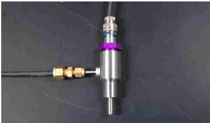
Figure 4.4. Custom Residual Gas Injector
