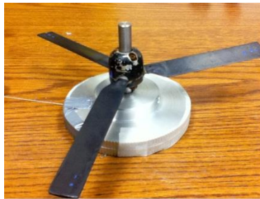
Figure 3.17. Vertical shaft with rotor referenced to zero
