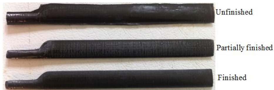
Figure 3.5 Manufactured composite blades
