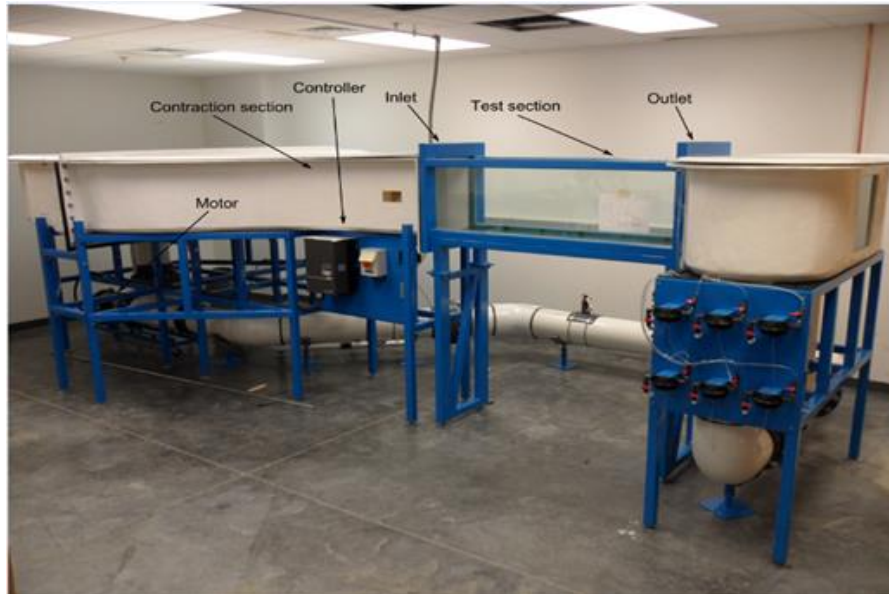
Figure 3.1. Water tunnel facility
