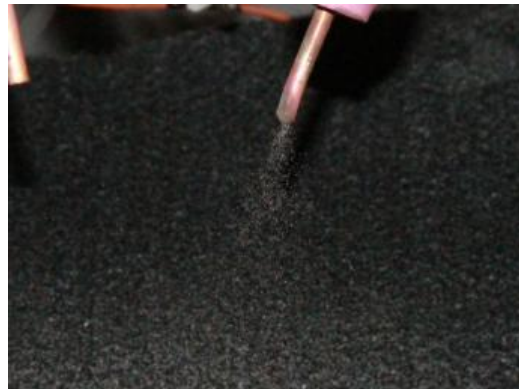
Figure 1.3 Powder stream from current powder feeding tube. The powder stream exits the copper nozzle in the center of the figure. The tube's outer diameter is 0.125".
