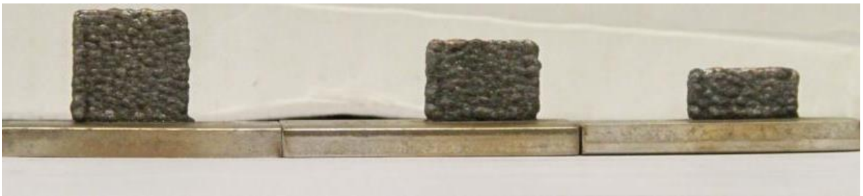
Figure 4.1 Parts made using the height control system. The part heights from left to right are 20mm, 15mm, 10mm.
