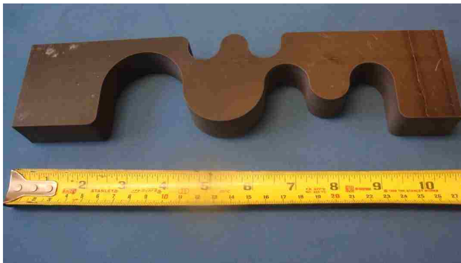
Figure 4.7. Coupon cut at 90,000psi at a traverse rate of 23ipm, AFR 1.5lbs/min, cutting head 0.013"/0.040"
