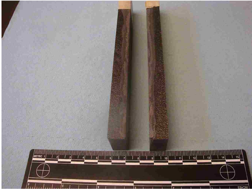
Figure 4.5. Bottom side erosion on a 1" thick composite sample
