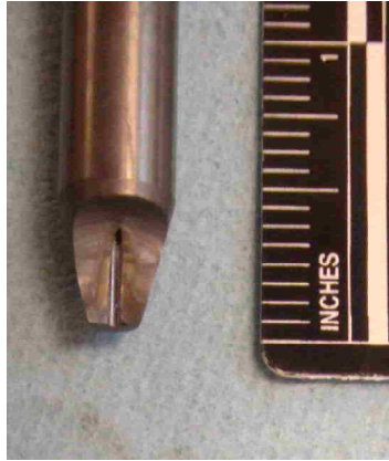
Figure 4.15. Damaged Focusing Tube
