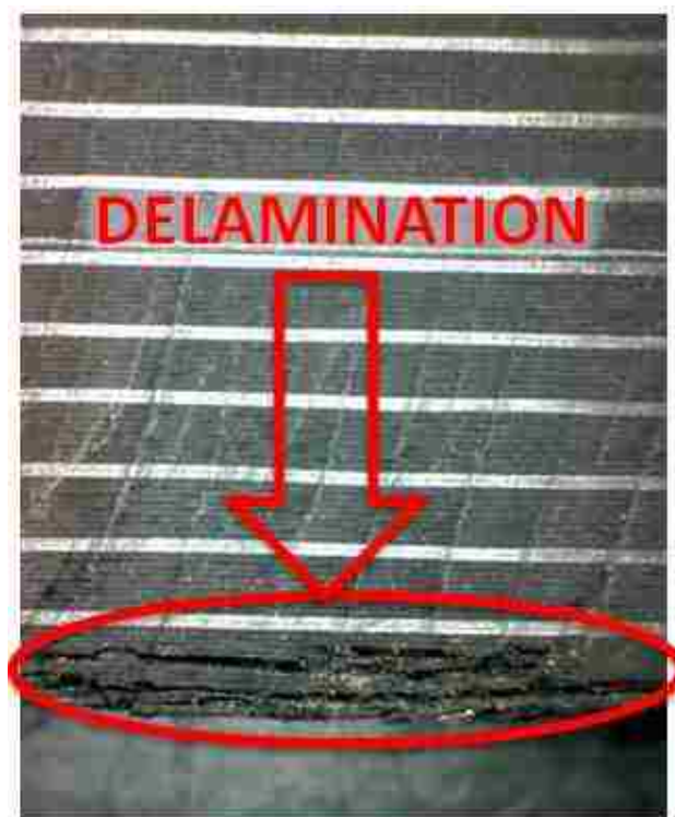
Figure 4.2. Delamination of 1" composite cut at 50,000psi (25x)
