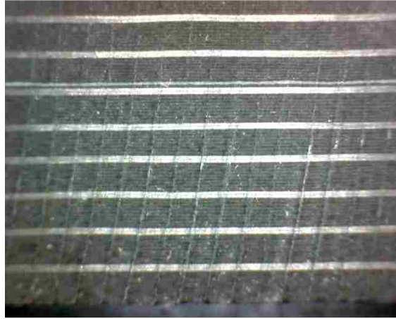
Figure 4.13. Jet striations on a sample (15x)
