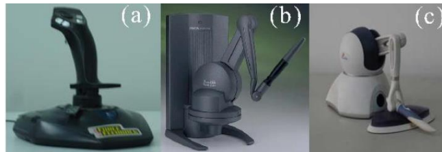
Figure 2.4 (a) force feedback joystick, (b) Phantom Desktop, (c) Phantom Omni [14]
