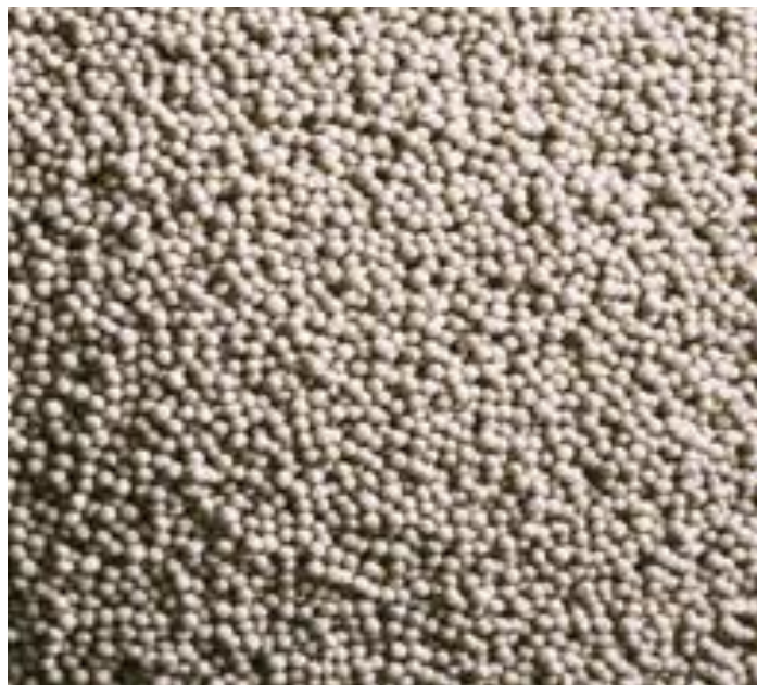
Figure 2.8. High strength traceable ceramic proppant (CARBO Ceramics)
