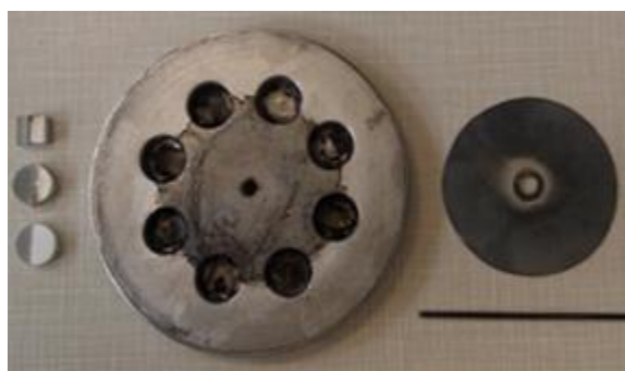
Figure 2.1 The magnetron sputtering target. The sputter material is replaced with the sample holder (left) with a shadow shield that covers half the exposed sample face (right).
