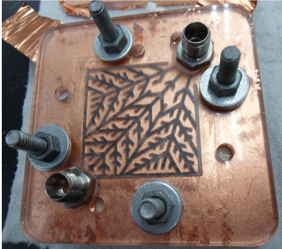
Figure 4.3 Assembled fuel cell with clear bipolar plates
