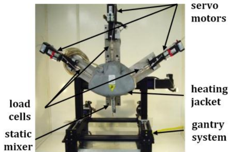
Figure 2.1. The triple-extruder Freeze-form Extrusion Fabrication (FEF) machine.
