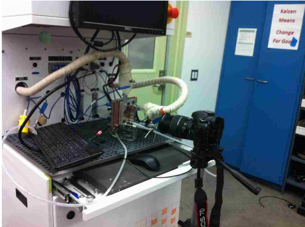
Figure 4.4 Fuel cell test setup for direct visualization with high resolution digital camera
