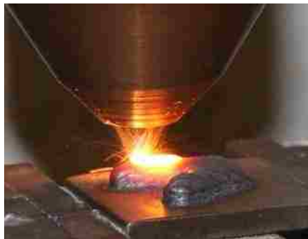
Figure 1.1 A blown powder metal deposition process is depositing a steel part
