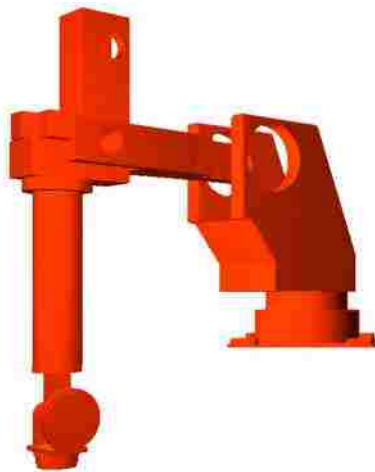
Figure 3.4 Robot's posture when joints value as [0^\circ \ 0^\circ \ 0^\circ \ 0^\circ \ 0^\circ \ 0^\circ]
