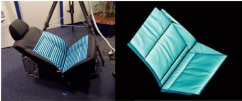
Figure.5.3 Structured light 3D scanner scanning a car seat to generate 3-D profile
